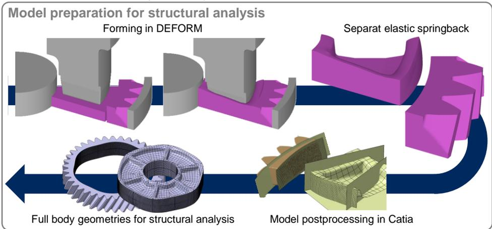
Figure. 3.2: Preparation of formed geometries for structural analysis
