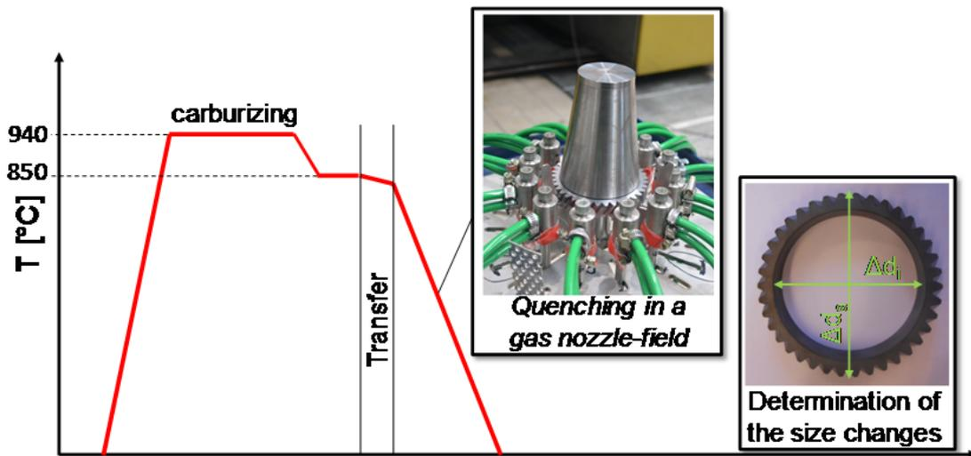
Figure 2.1: Schematic representation of the process chain "joining during quenching"
