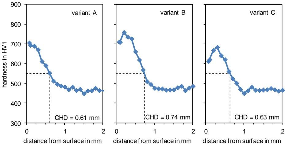
Figure 6: Hardness profile and CHD<sub>550</sub> in the case-hardened layer of the three variants
