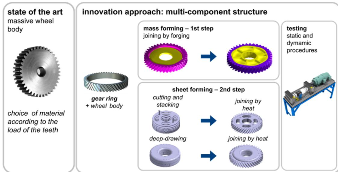
Figure 1.1: Design approach for multi-component gears
