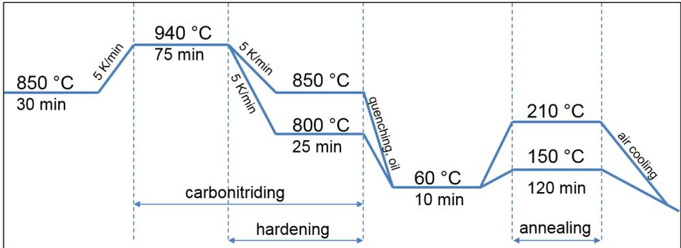
Figure 1: Time-temperature profiles utilized in carbonitriding of the specimen and test gears
