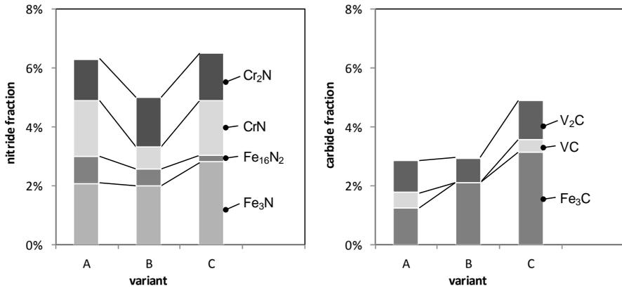
Figure 5: Phase fraction of different nitrides and carbides, measured at 100  $\mu\text{m}$  distance from the surface
