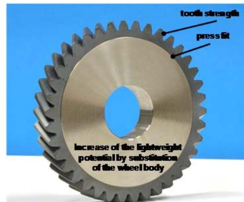
Figure 4.1: During heat treatment joint gear and tasks for further investigations
