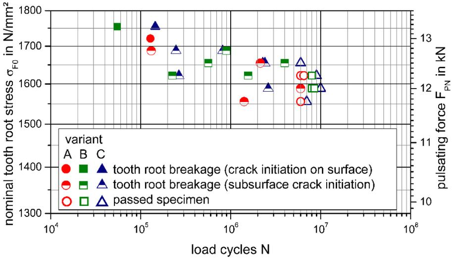
Figure 7: Tooth root bending test results for Variants A, B and C
