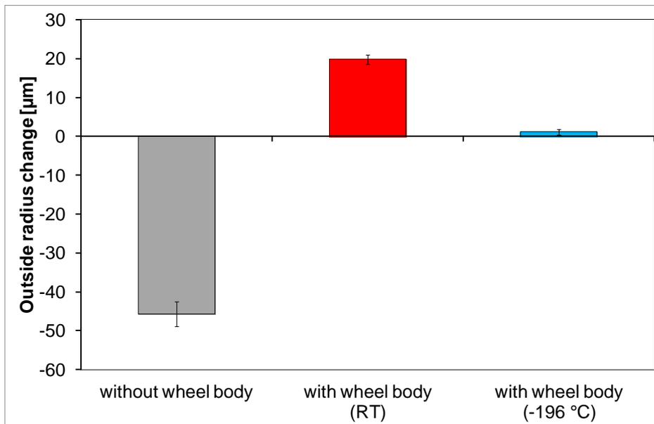
Figure 3.2: Outside diameter changes of the freely quenched and joint gear ring (CHD 0.5 mm)
