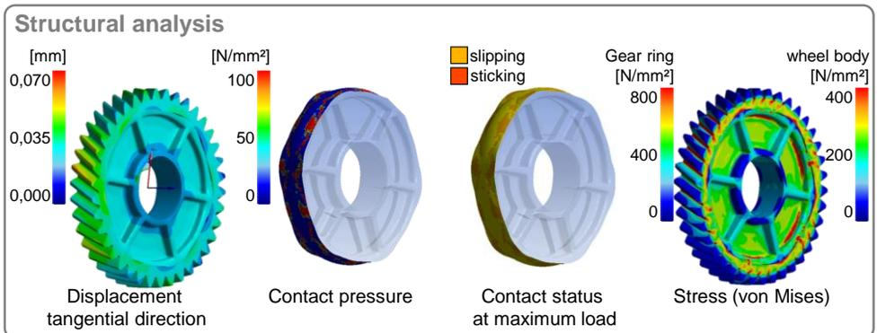
Figure. 4.4: Illustration of the numerical model in Ansys, contact and stress results at 400 Nm torque
