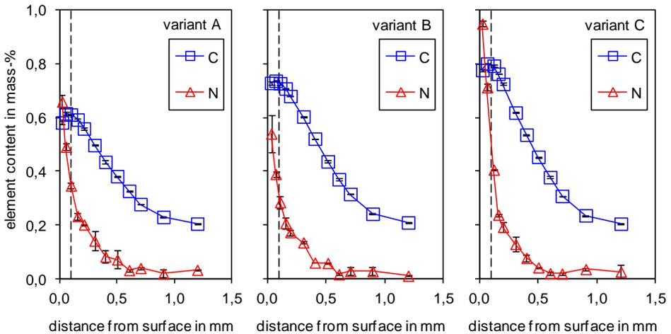
Figure 2: Carbon and nitrogen distribution in the case-hardened layer of the three variants, broken line indicates 100 μm distance from the surface
