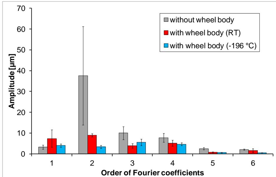
Figure 3.3: Distortion of the outer diameter; Fourier spectra
