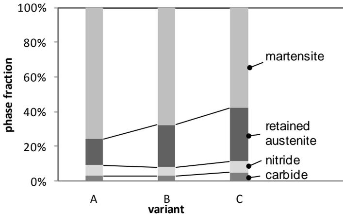
Figure 4: Phase fraction of martensite, retained austenite, nitrides, and carbides, measured at 100 µm distance from the surface
