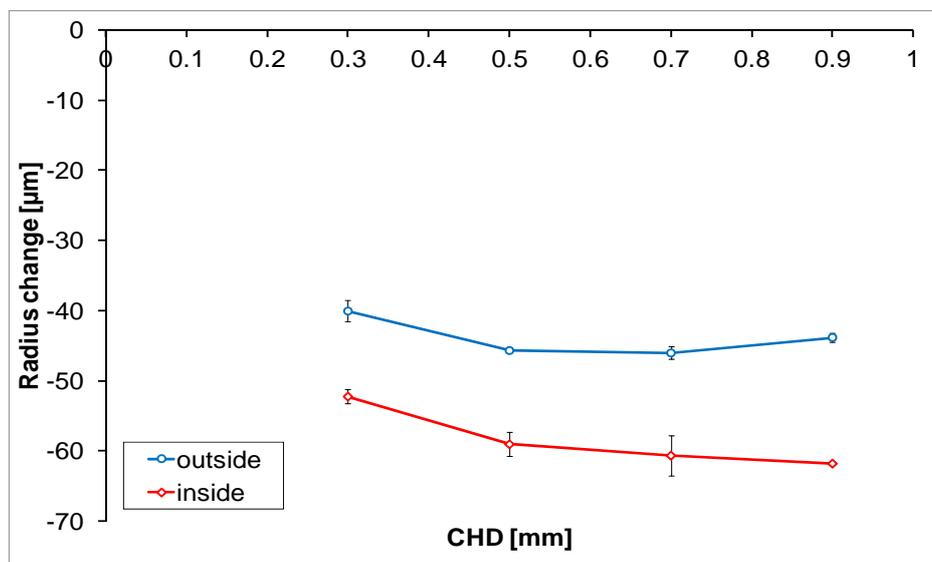
Figure 3.1: Influence of the CHD on the outside and inside radius change of the gear rings
