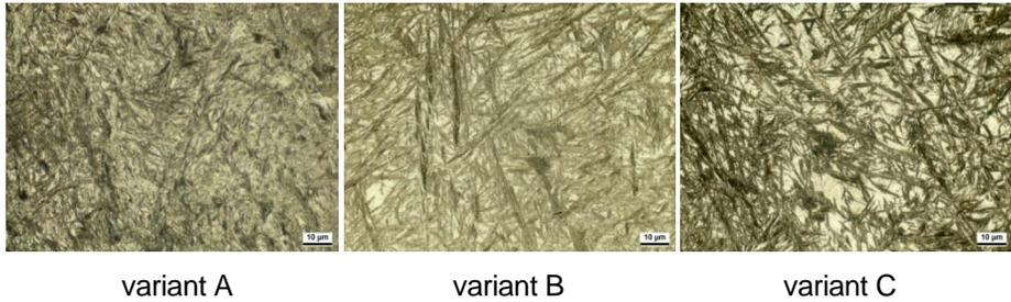
Figure 3: Microstructure of the carbonitrided steel after heat treatment (etching: 35 s, 3% alk. HNO<sub>3</sub>; sampling: longitudinal), taken at 100 µm distance from the surface
